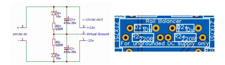
24v DC Supply split into +12v and -12v | D2+, D2-, R2+ and R2- on PCB
